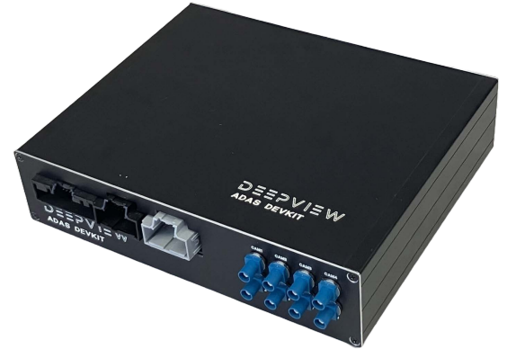
AI Vehicle Computer featuring Nvidia Orin AGX
