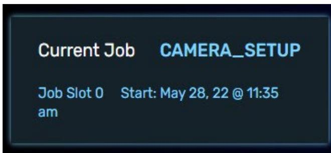
By default, the job is CAMERA\_SETUP, which is used to capture images prior to training.
