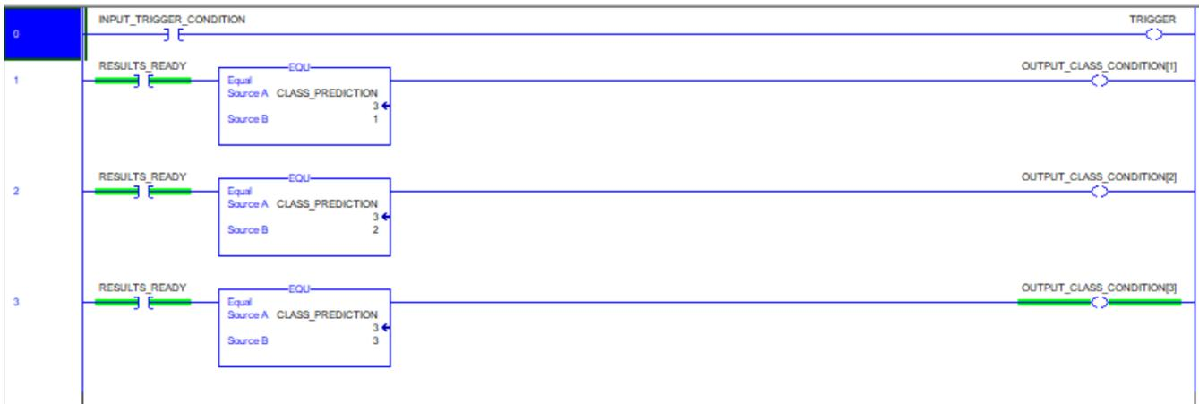
The image above is an example of a PLC program written to run a classification job. **CLASS\_PREDICTION** is a DINT set by the camera.
