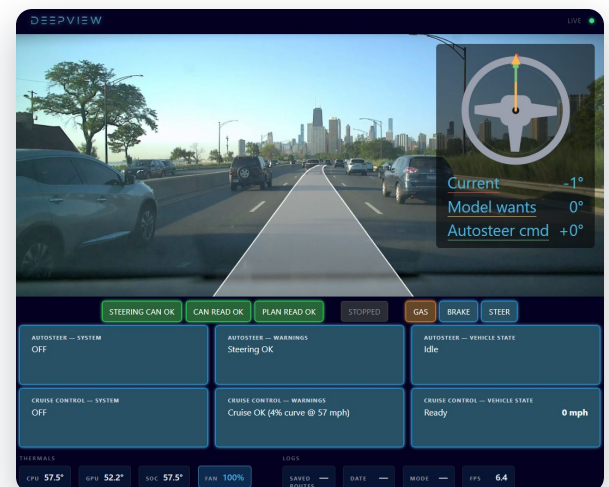
X2000 development UI — live camera with path overlay, steering intent, and vehicle state
